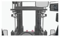
**Optimized Design for Wide Vision Mast:** The new forklift features a wide vision mast design that ensures the operator has a better view during operation, reducing blind spots and enhancing safety.
